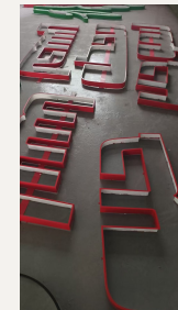
Fabricated hollow returns / structure before assembly
