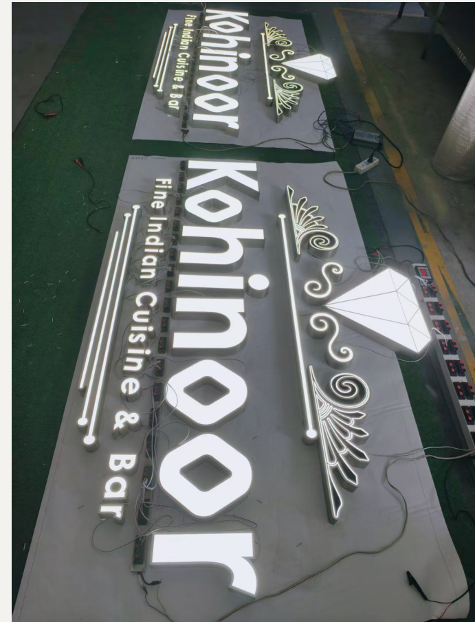
Assembled sign / illumination check
